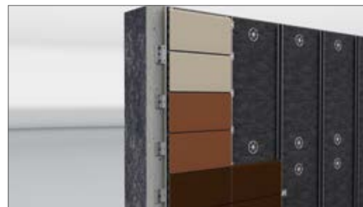
Mount the KeraTwin® panels in vertical rows
